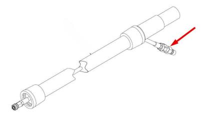
2. Remove the filter cartridge and orifice plate, place them in a cup of white vinegar and soak for 30 minutes.
