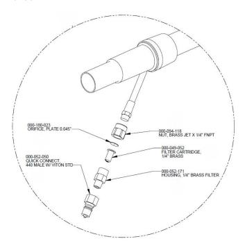
3. Clean the orifice plate's opening with a wooden skewer or a similar non-metallic tool.
