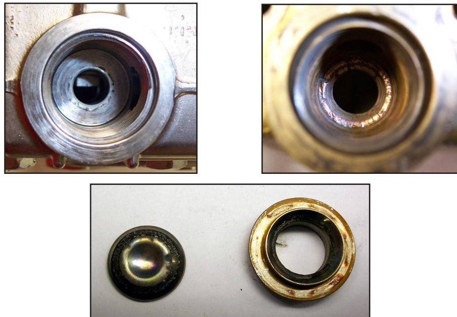
Figure 5-2. Inspect Manifold and Old Valves
