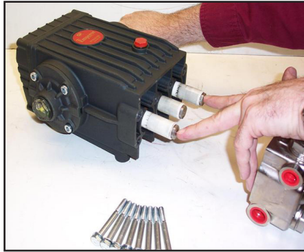
Figure 5-16. Re-install Manifold and Torque Fasteners
