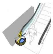
The unique swivel mount allows the cart to clean handrails directly next to walls or other obstacles
