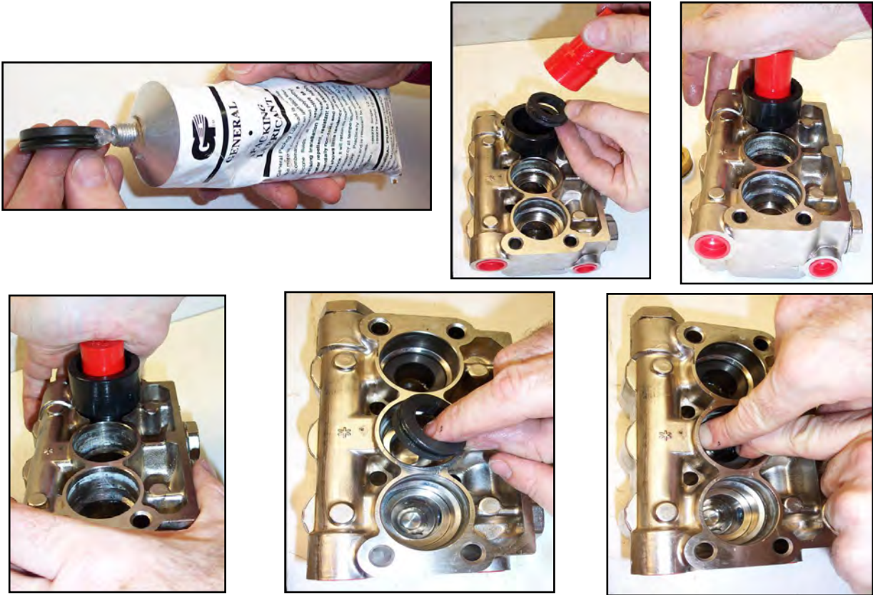
Figure 13. Install Seal Assembly Using O-Ring Grease
