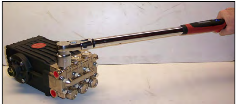
Figure 5. Replace Valve Cap and Torque to 95 ft. lbs.
