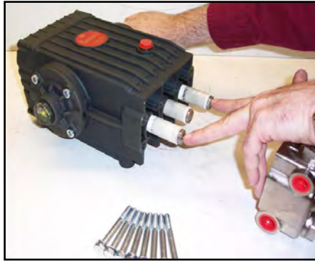
Figure 16. Re-install Manifold and Torque Fasteners
