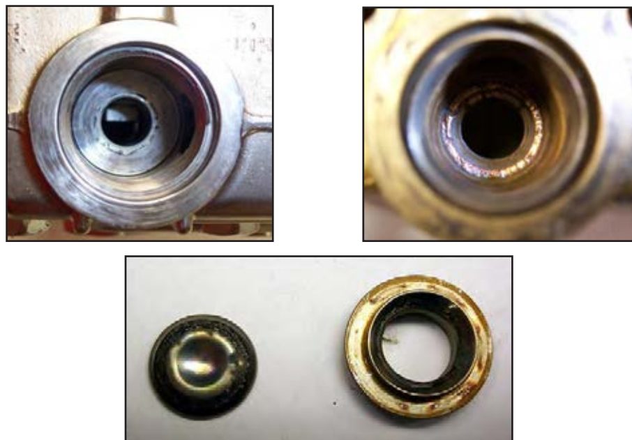
Figure 5-2. Inspect Manifold and Old Valves
