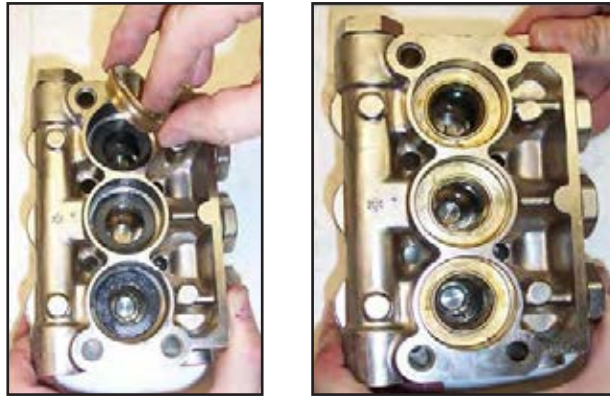
Figure 5-14. Install Retainers into Cavities
