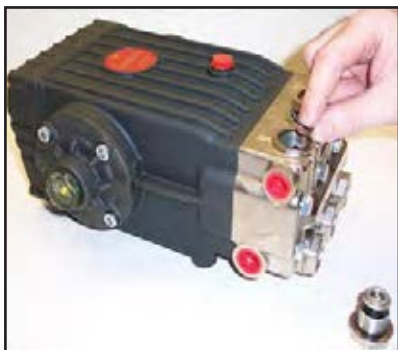
Figure 5-4. Apply Grease and Install Valves
