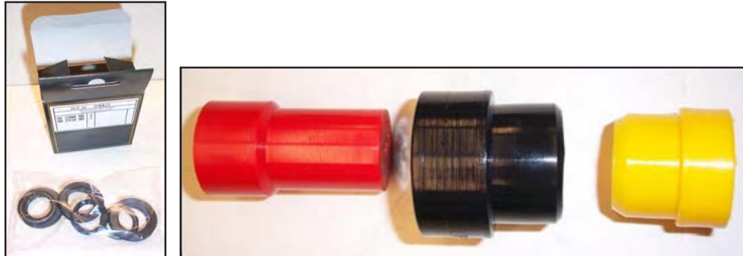
Figure 5-12. Seal Kit and Insertion Tool for Seal Installation
