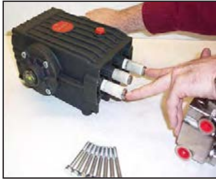
Figure 5-16. Re-install Manifold and Torque Fasteners
