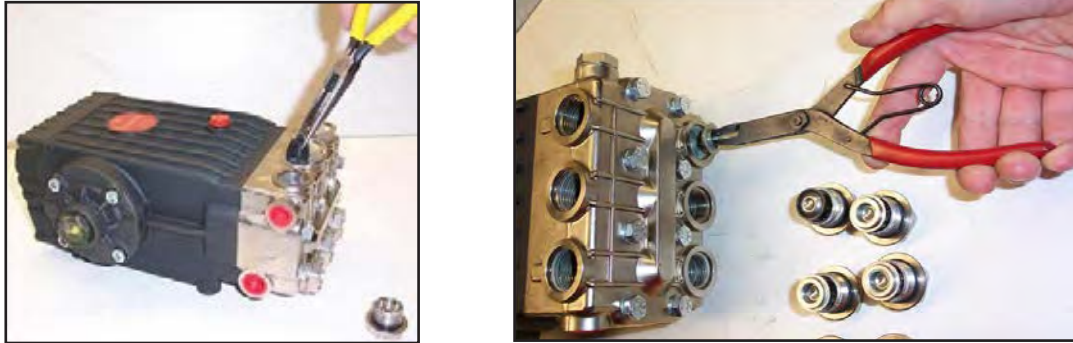
Figure 5-1. Remove Valve Cap and Valve Assembly
