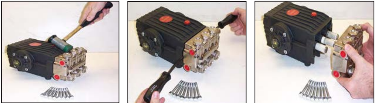
Figure 5-6. Separate Manifold from Crankcase
