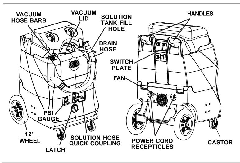
**SWITCH PLATE** - The switches are located on the rear of the machine, out of the way of water **FAN** - Removes warm air from the component compartment.
