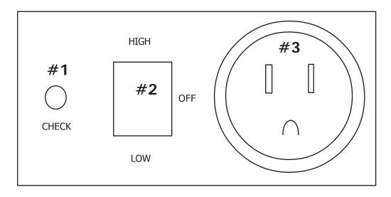
CHECK FILTER LIGHT (1): This light will come on when the filters are loaded and need to be replaced. Always check the light with the switch on the HIGH setting. Turn the machine off to change filters.
