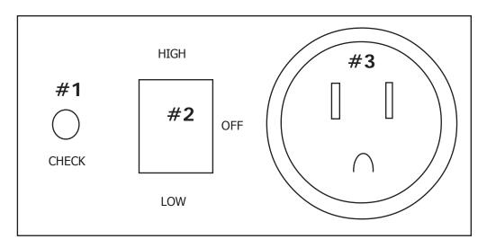
**CHECK FILTER LIGHT (1)**: This light will come on when the filters are loaded and need to be replaced. Always check the light with the switch on the HIGH setting. Turn the machine off to change filters.
