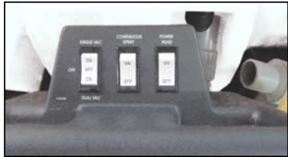
Figure 4. Ensure All Switches are in the OFF Position
