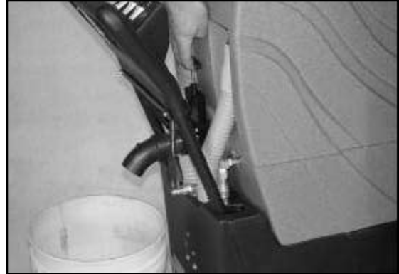
Figure 15. Draining Recovery Tank
