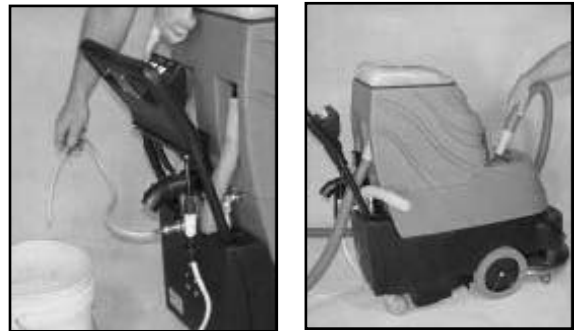
Figure 16. Draining Solution Tank
