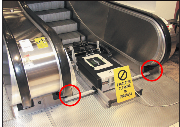
Figure 13. Ensure Restraining Arms are Firmly Seated Against Balustrades
