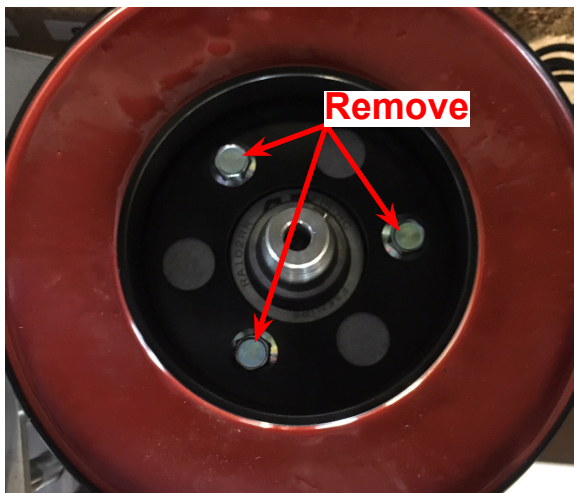
Figure 31a. Preparing the Clutch Assembly
