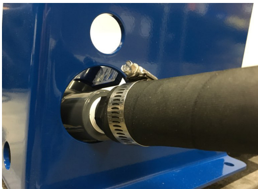
Figure 70. Attaching 6" Hose to the Valve
