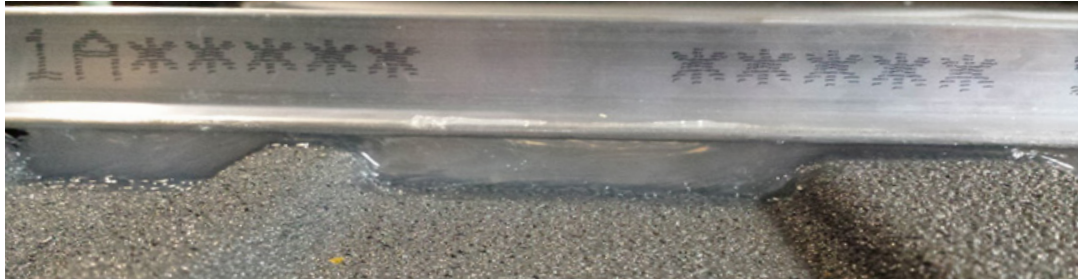
Figure 5. Application of Silicone Between the Angle and the Van's Floor
