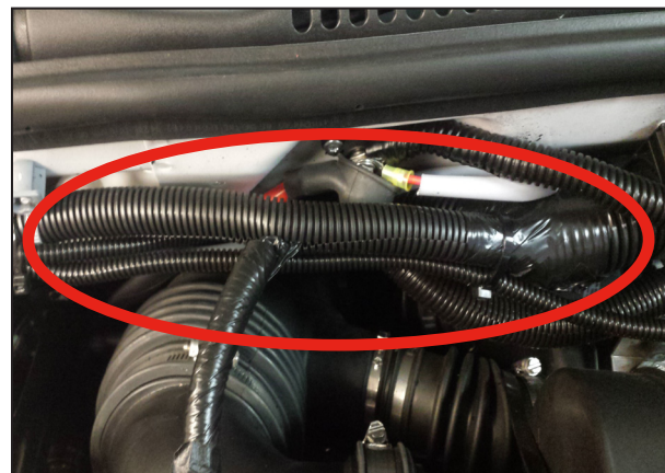
Figure 38. Hold Main Wire Harness Away from CDS Clutch
