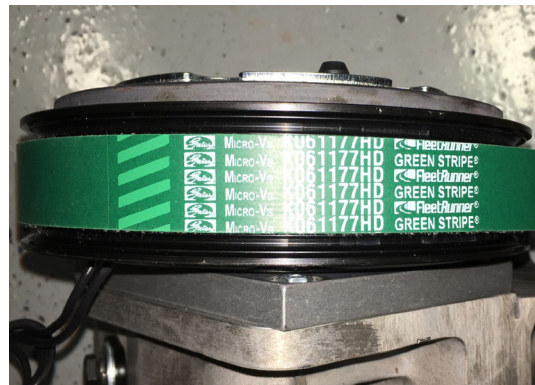
Figure 36. Center the Belt on the Pulley by Leaving One Groove Empty on Each Side
