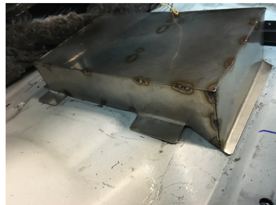
Figure 18. Lower New Cover over SDM and Sensor
