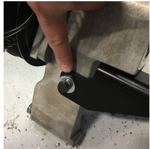
Figure 31. Grounding location on the clutch housing
