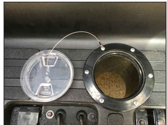
Figure 56. Secure with 6 Self-Tapping Screws
