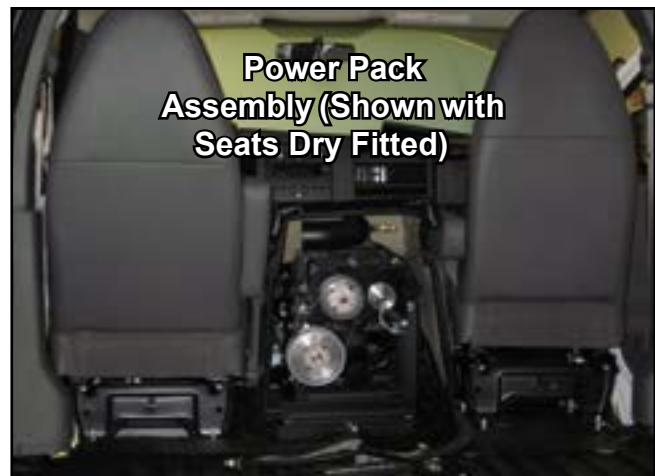
Figure 38. Dry Fit Vehicle Seats and Power Pack
