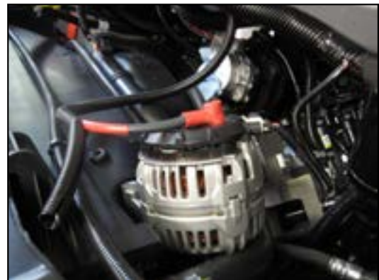
Figure 15. Attach New Battery Cable
