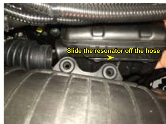
Figure 29. Slide Resonator Off Hose; Remove Resonator from under Hood
