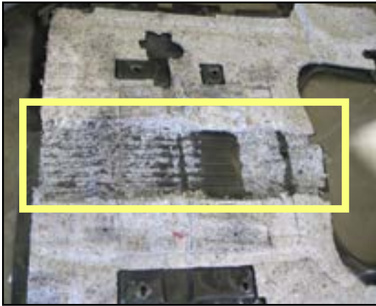
Figure 10. Remove Batting from Floor Mat
