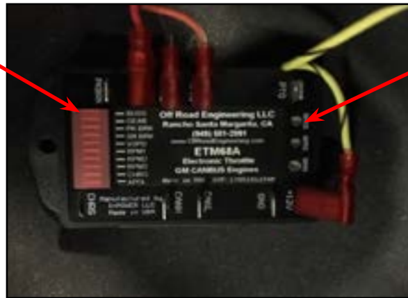
Figure 59. Location of Controller's LED Lights with Labels and RPM Trim Potentiometers
