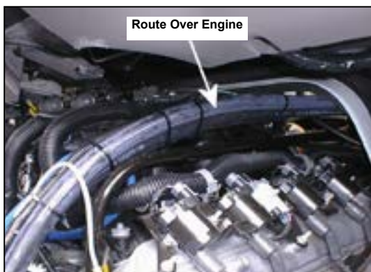
Figure 25. Secure Hoses with Provided Clamps
