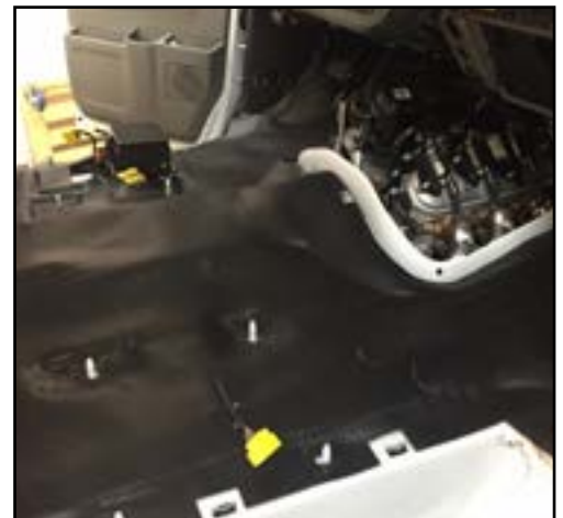
Figure 12. Finish Yaw Sensor with front mat reinstalled
