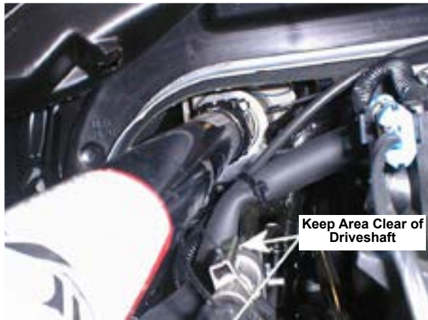
Figure 39. Slide Yoke into Drive Shaft
