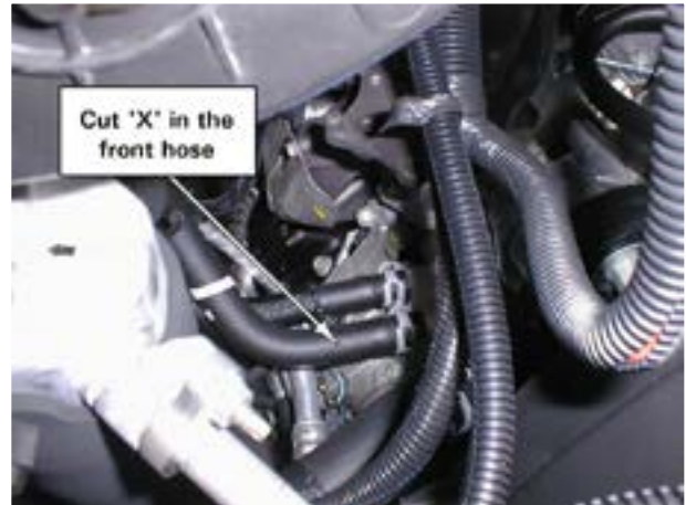
Figure 23. Cut Small 'x' in Water Pump Hose
