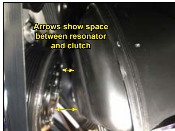
Figure 33. Note Space between Resonator and Clutch
