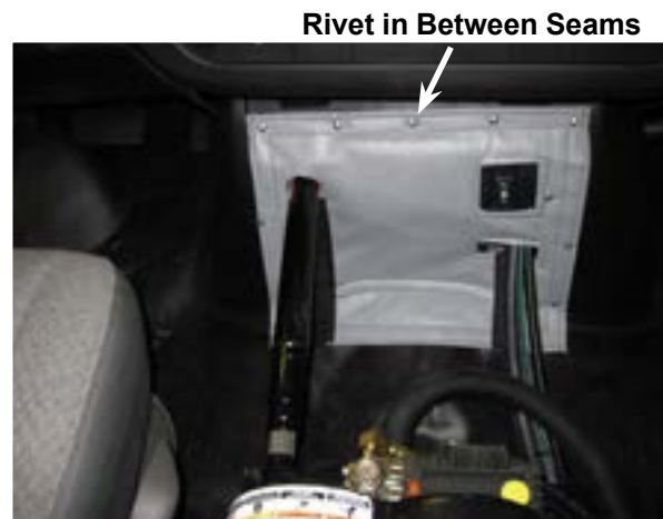
Figure 56. Position Seal as Shown
