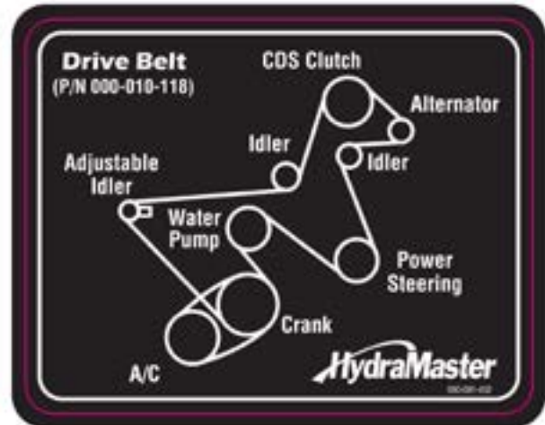
Figure 20. Routing Diagram for Drive Belt
