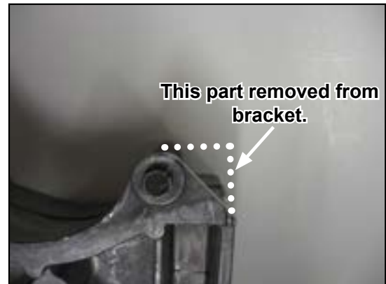
Figure 16. Remove Top Right Corner of Bracket
