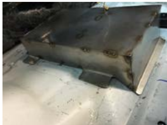
Figure 7. Lower New Cover over SDM and Sensor
