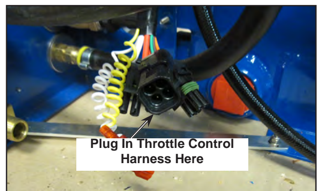
Figure 38. Connect Throttle Control Harness to 4 Pole Plug
