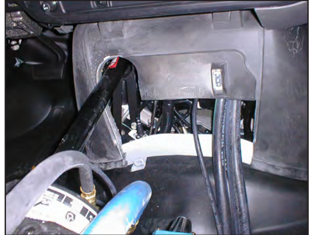
Figure 58. Fit Over Pump and Hoses
