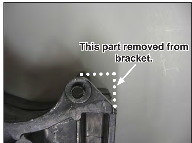
Figure 16. Remove Top Right Corner of Bracket
