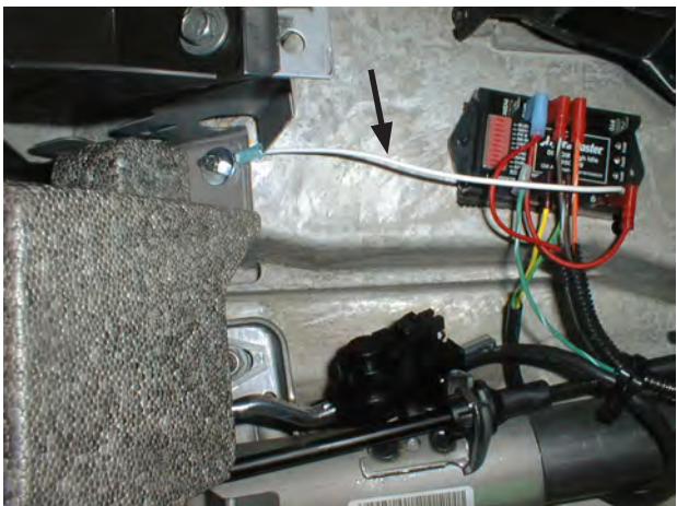
Figure 34. Connect White Wire to Ground
