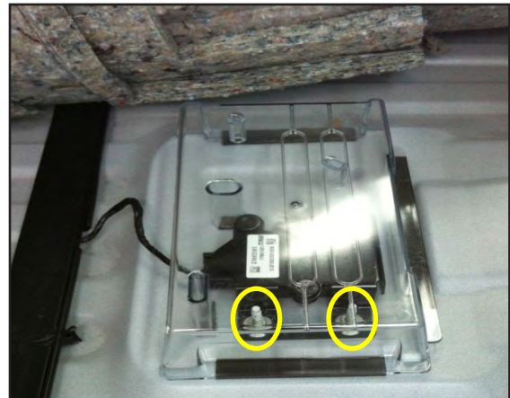
Figure 5. Remove the Original Clear Plastic Cover Remove
