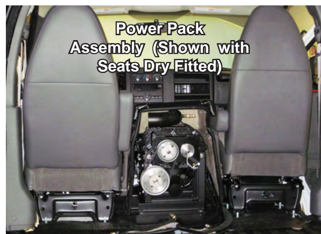
Figure 40. Dry Fit Vehicle Seats and Power Pack
