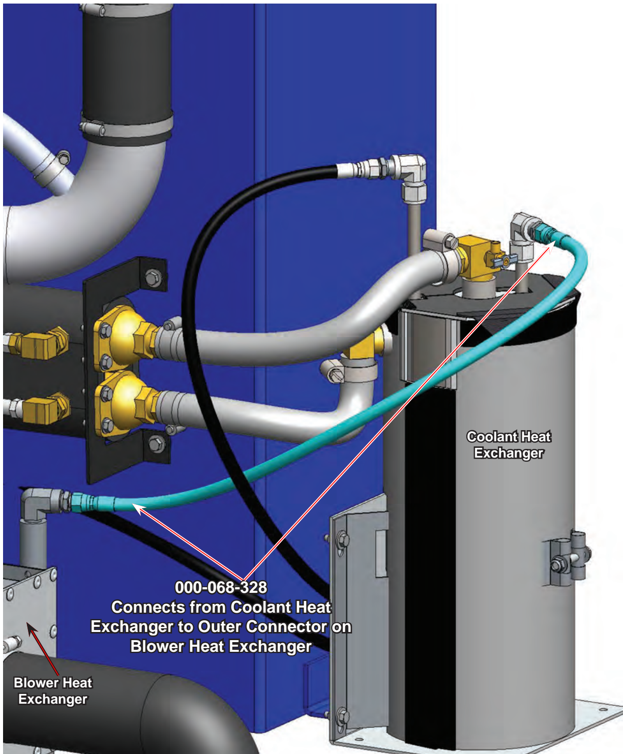
Figure 83. Route and Connect Hose from Coolant Heat Exchanger to Outer Connector on Blower Heat Exchanger
