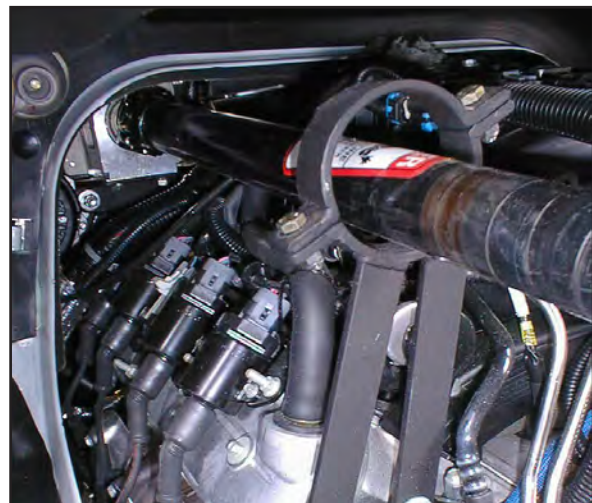
Figure 20. Install Safety Ring
