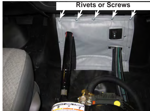
Figure 59. Position Seal as Shown
