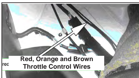
Figure 37. Route Throttle Cable to Controller
