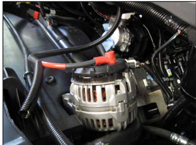
Figure 15. Attach New Battery Cable
