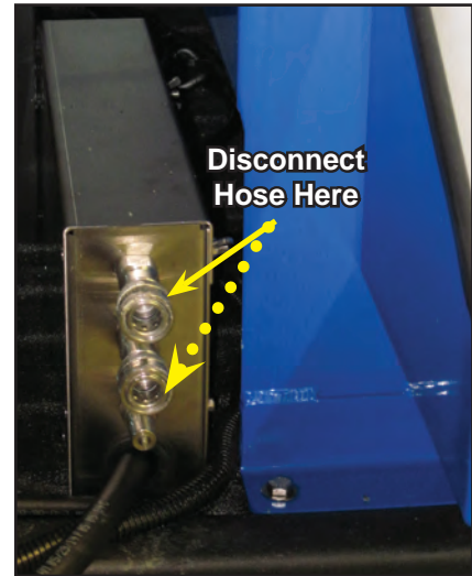
Figure 98. Disconnect Solution Hose
