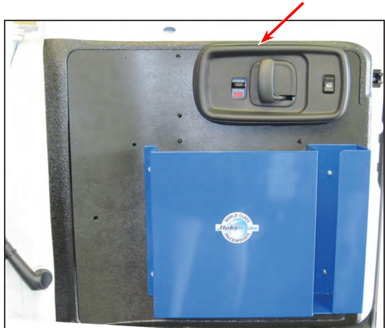
Figure 103. Install Trimlok (P/N 000-131-060) Around Door Handle
