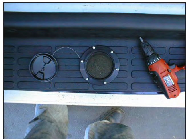
Figure 49. Secure with 6 Self-Tapping Screws
