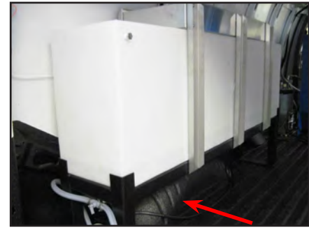
Figure 67. 50 Gallon Tank Assembly Positioned Over Wheel Well
