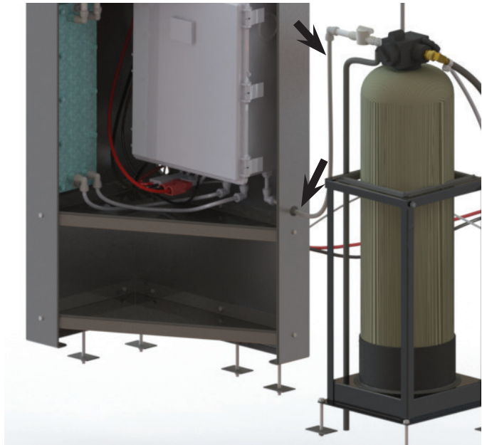
Figure 88. Route Tube through EWS Shelf to Connector on Electrical Box
