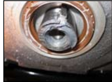
Figure 34. Sealant MUST Be Secured within 4 Minutes
