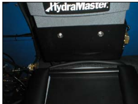
Figure 30. Water Box and Cowling Should Barely Touch
