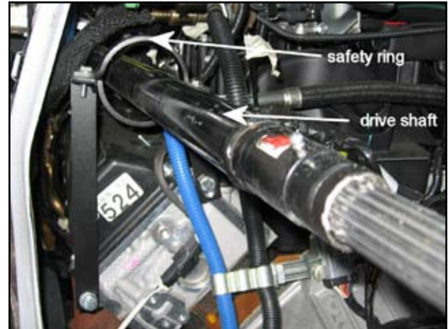
Figure 19. Driveline Should Not Contact Safety Ring
