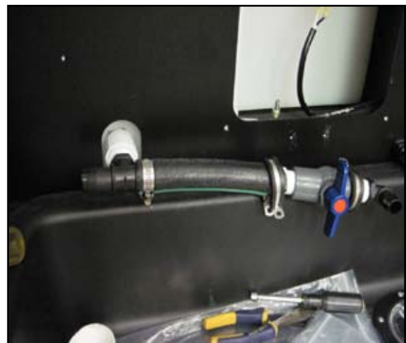
Figure 28. Install Drain Hose and Valve
