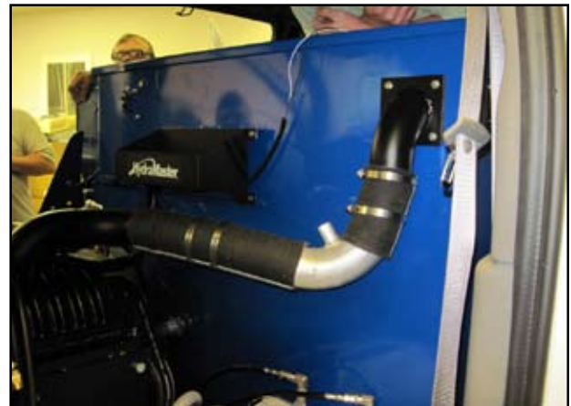
Figure 14. Install Hoses and Elbow onto Recovery Tank
