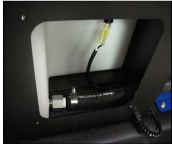
Figure 27. Route Hose from Water Pump through CDS Console
