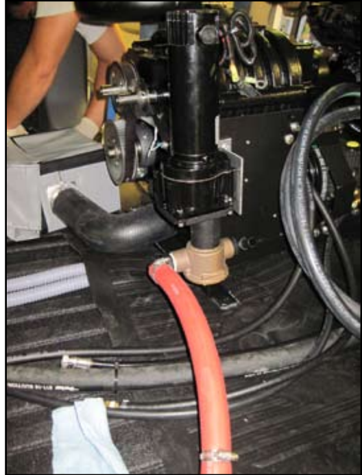
Figure 5. Install APO onto Power Pack
