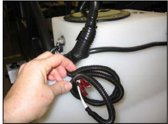
Figure 31. Float Wire Connectors
