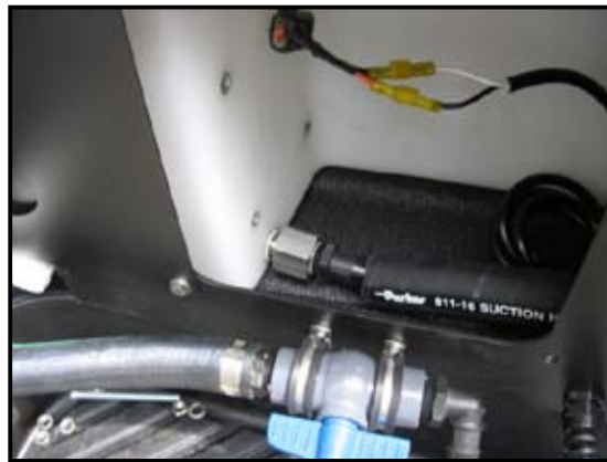
Figure 33. Remove Front Access Panel and Route Through Tank
