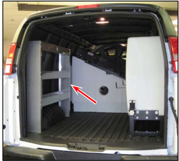
Figure 37. Secure Stainless Steel Shelf to Van's Wall and Floor
