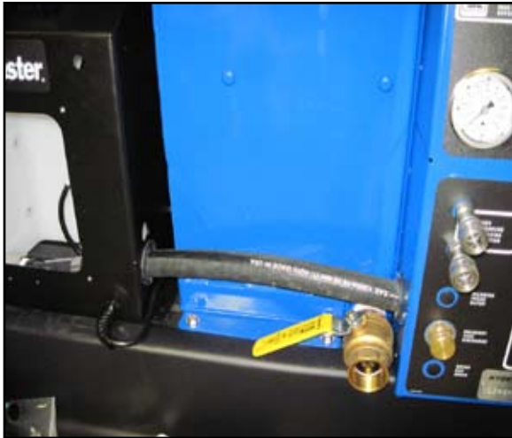
Figure 27. Route Hose from Water Pump through CDS Console
