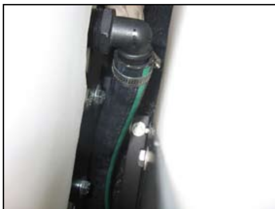
Figure 35. Connect Pump Hose to 110 Gallon Tank
