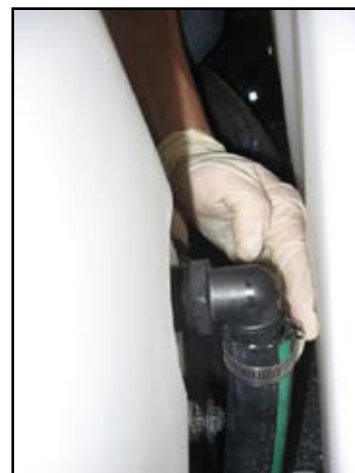
Figure 35. Connect Pump Hose to 110 Gallon Tank
