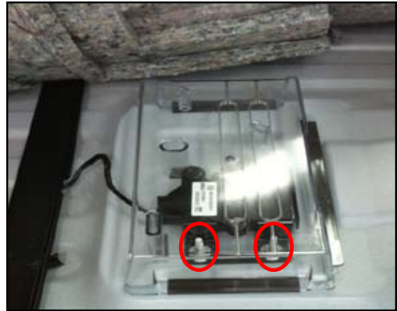
Figure 2. Remove the Original Clear Plastic Cover
