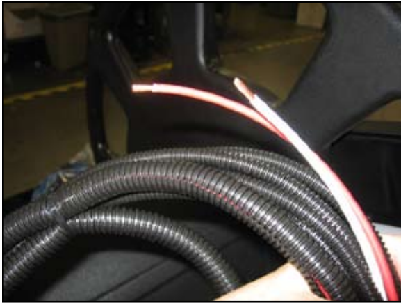
Figure 30. Battery Cables without Connectors
