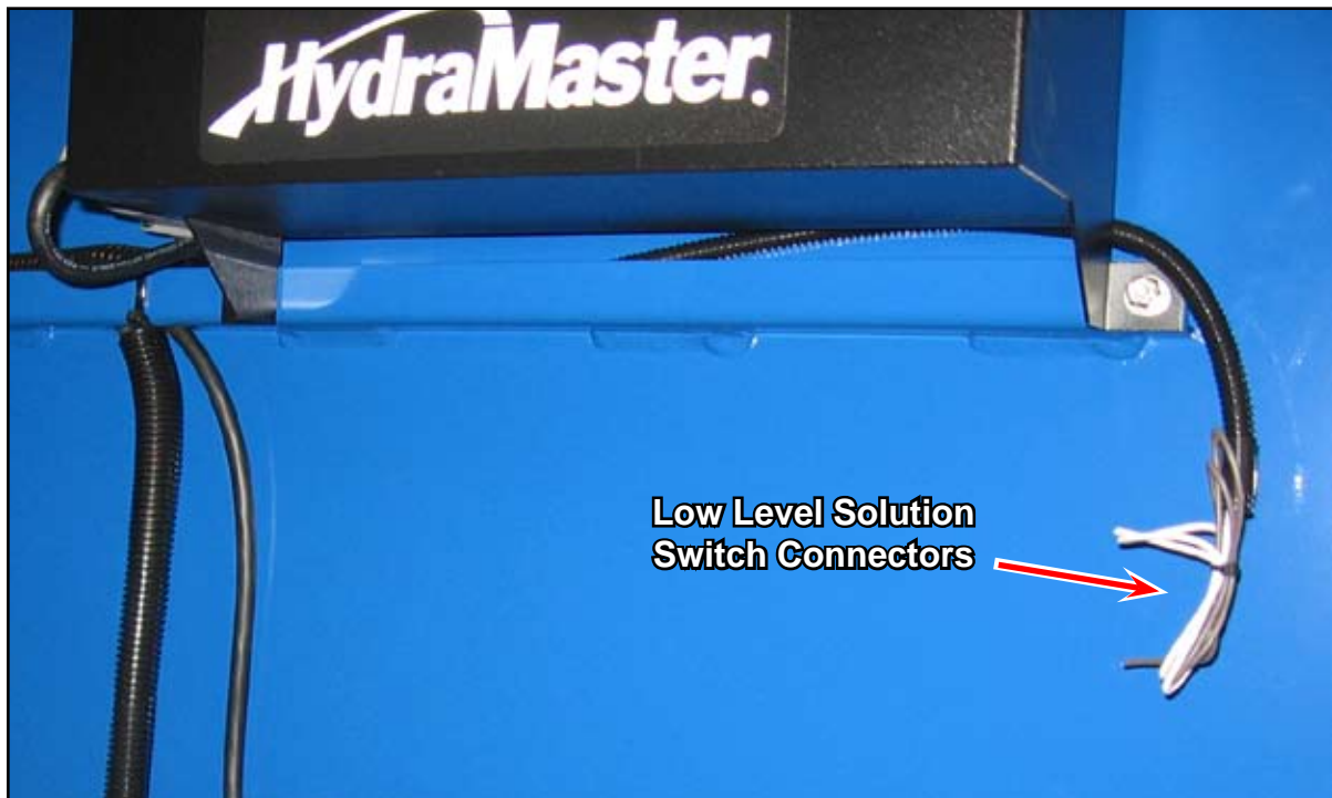
Figure 32. Attach Float Wire Connectors from HydraCradle Tank to CDS' Low Level Solution Switch Connectors
