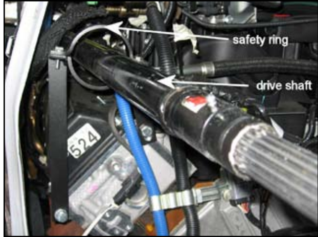
Figure 19. Driveline Centered in Safety Ring
