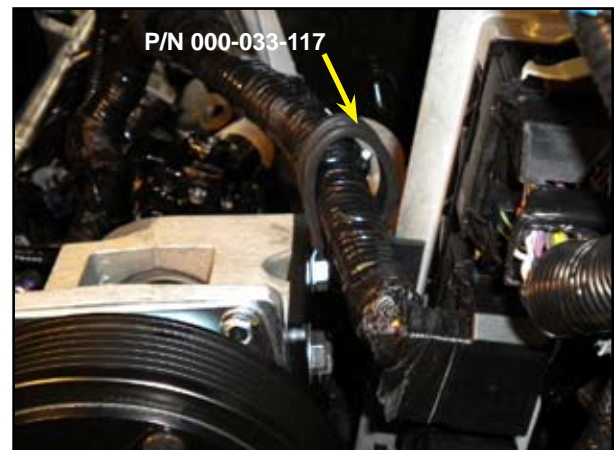
Figure 13. Install 1" Clamp and Route Larger Harness
