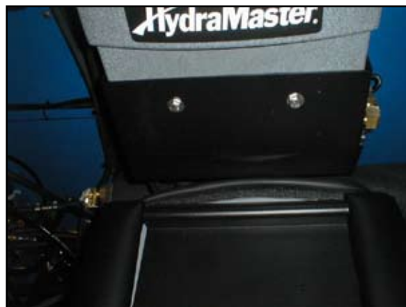
Figure 31. Water Box and Cowling Should Barely Touch
