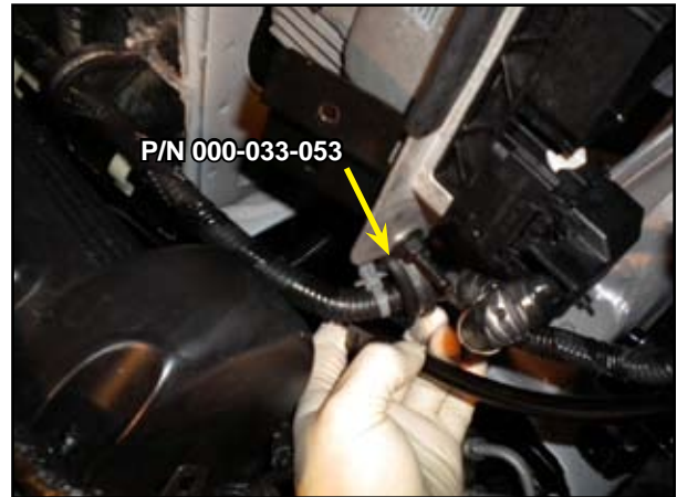
Figure 11. Route Smaller Harness, in Lower Position, using One P/N 000-033-053 Clamp (1 1/2")
