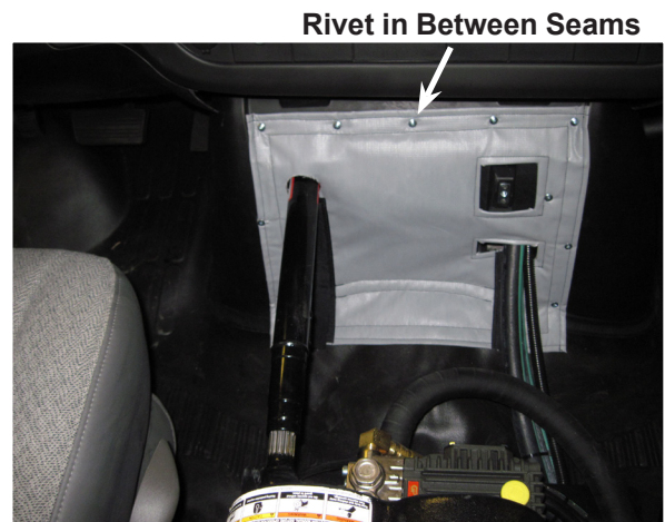
Figure 54. Position Seal as Shown
