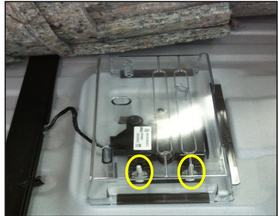
Figure 4. Remove the Original Clear Plastic Cover
