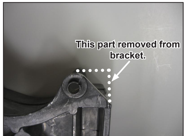
Figure 15. Remove Top Right Corner of Bracket
