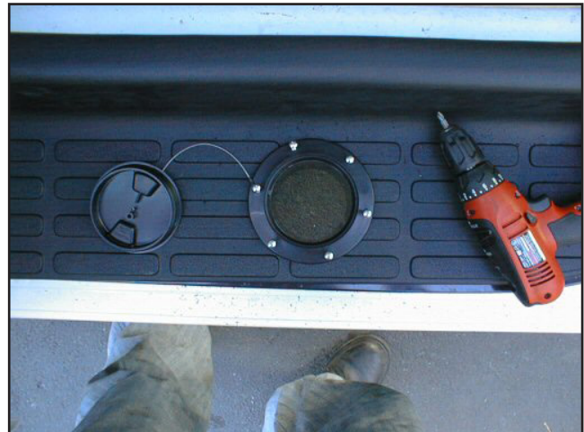
Figure 51. Secure with 6 Self-Tapping Screws
