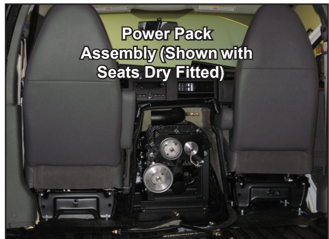
Figure 28. Dry Fit Vehicle Seats and Power Pack
