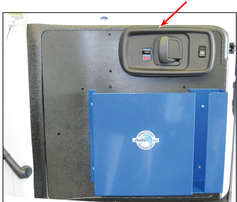
Figure 49. Install Trimlok (P/N 000-131-060) Around Door Handle
