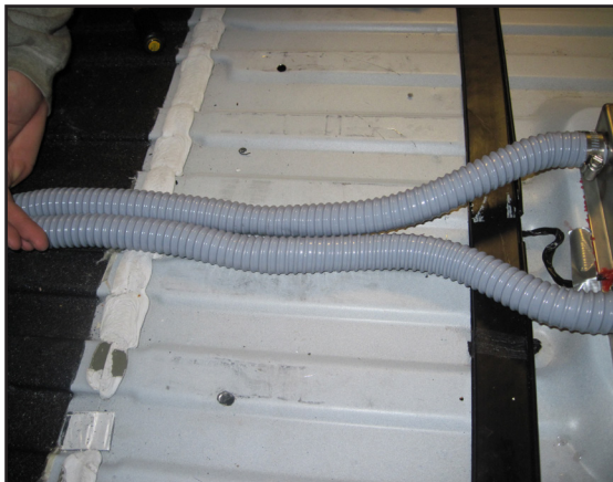
Figure 11. Route Hoses Straight Back Toward Cargo Area
