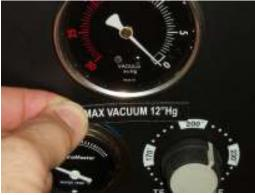
Verify that the vacuum level is set at 12" Hg. Adjust the vacuum level as necessary with the vacuum relief valve located on the recovery tank.
