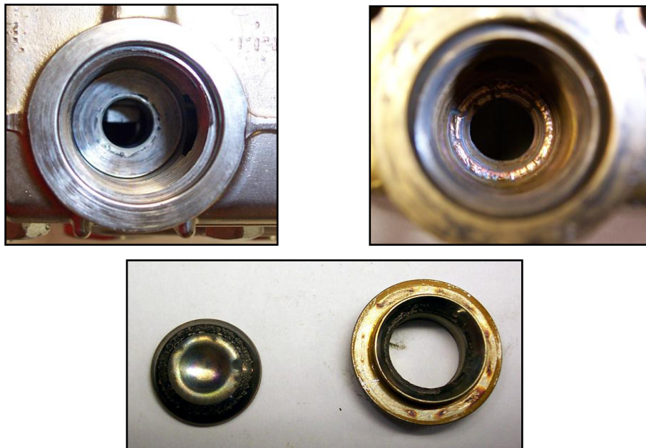
Figure 5-2. Inspect Manifold and Old Valves
