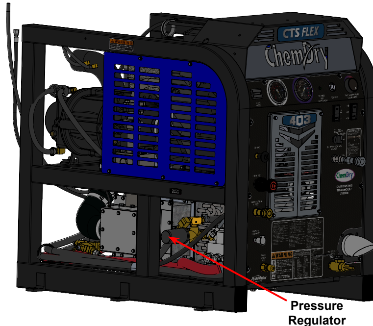
Figure 2-4. Side View of CTS 403 Flex Console
