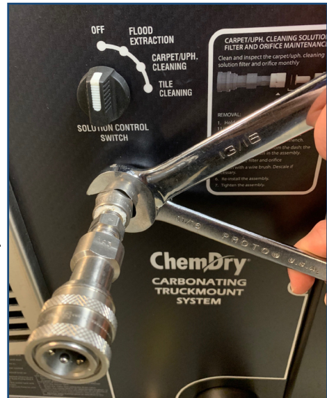
Figure 4-6. Remove Quick Connect Assembly
