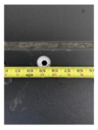
Drill out the octagon holes that correspond to the mounting rail holes to 9/16" with a step drill.
