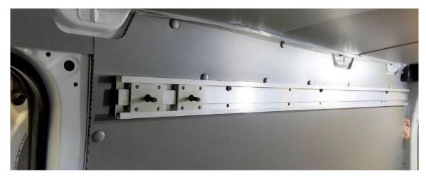
Mount the bottom rail in the same manner as the top rail only using the bottom set of holes.
