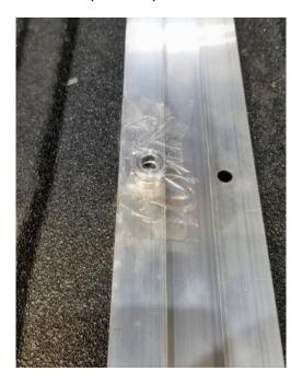
Two spacers may be required if the van has insulation on the side panels.
