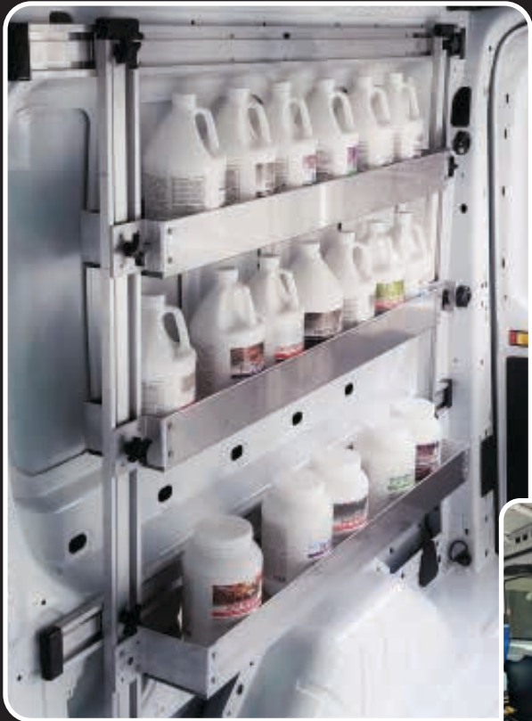
WAND STORAGE OPTION SHELVES CAN BE ADJUSTED WITH 2 OR 3 BINS WITH WAND
