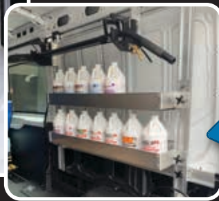
WAND STORAGE OPTION SHELVES CAN BE ADJUSTED WITH 2 OR 3 BINS WITH WAND
