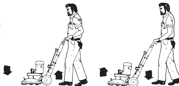
Figure 4-2. PowerHead Maneuvers Like a Buffer
