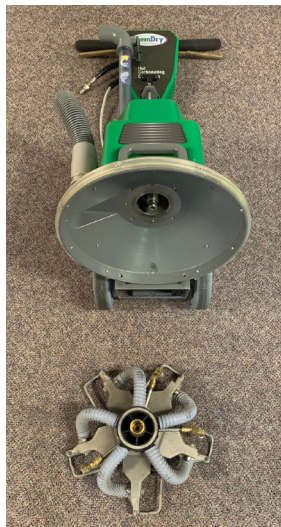
Figure 6-6. Removing the Star Assembly before Transport
