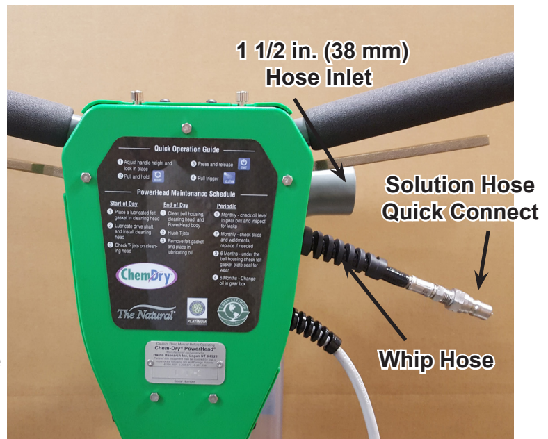
Figure 4-1. Solution and Vacuum Hose Connections
