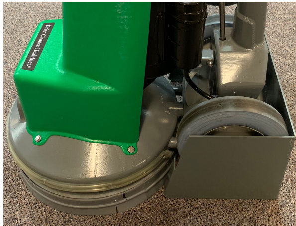
Figure 6-8. Properly Stored Unit in the Storage Bracket
