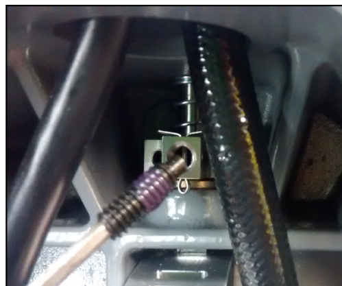
Figure 9-5. Reinstall dog point set screw
