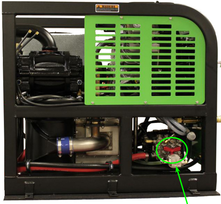
Chemical Pump Shutoff Valve
