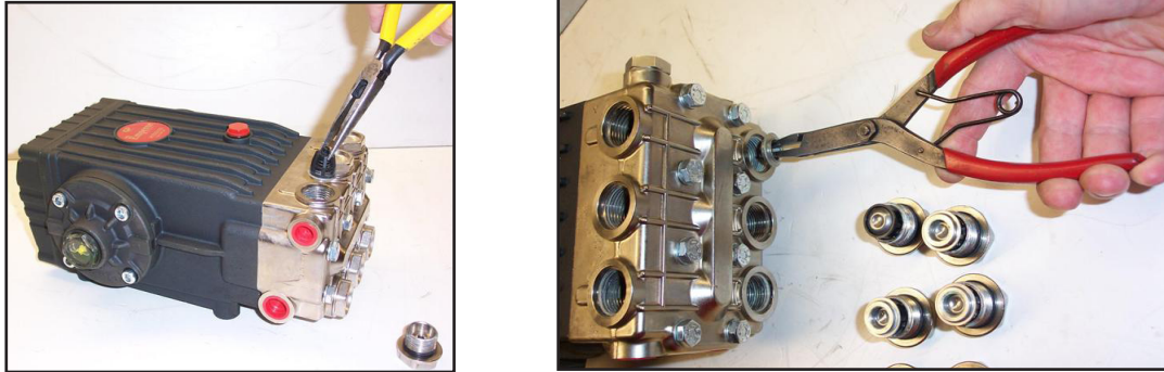
Figure 5-1. Remove Valve Cap and Valve Assembly
