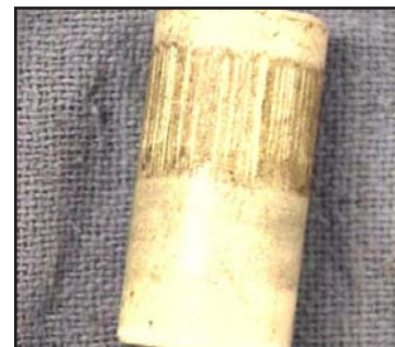
Figure 5-8. Examine Ceramic Plungers
