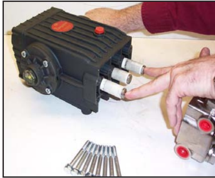
Figure 5-16. Re-install Manifold and Torque Fasteners
