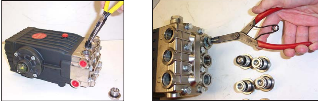
Figure 5-1. Remove Valve Cap and Valve Assembly
