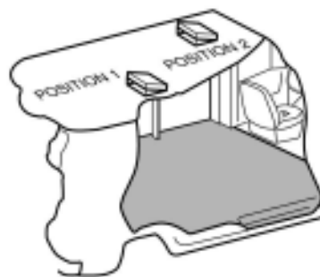
Figure 1-1 Roof Vent Locations
