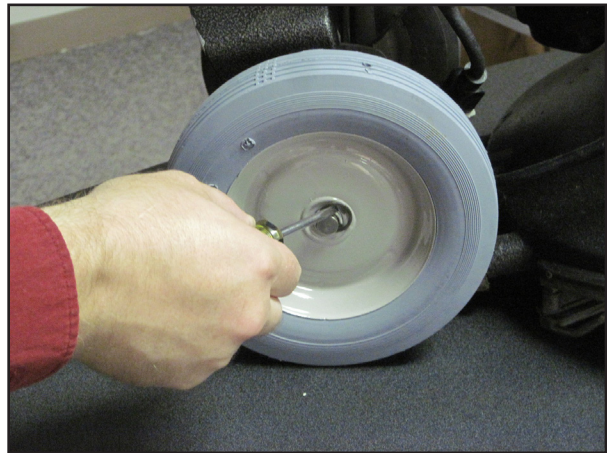
Figure 6-8. Remove Retaining Clip with Screwdriver
