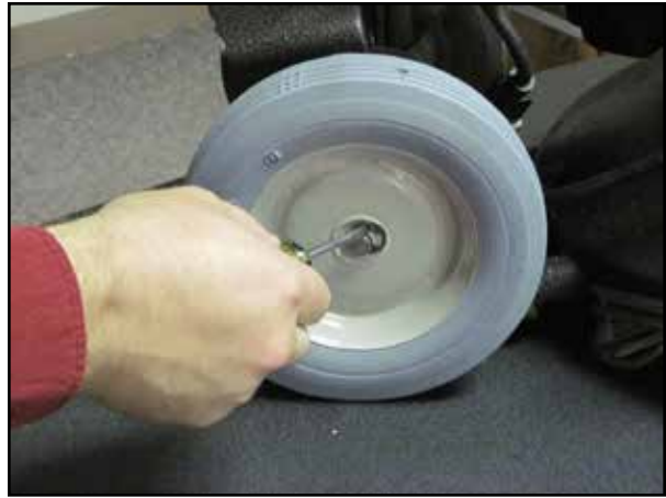
Figure 6-6. Remove Retaining Clip with Screwdriver
