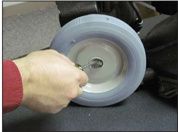
Figure 6-6. Remove Retaining Clip with Screwdriver
