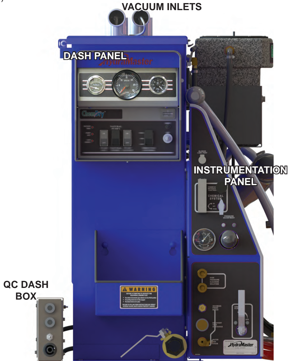
Figure 2-1. CTS 4.8 Flex Dash Panel and Instrumentation Panel
