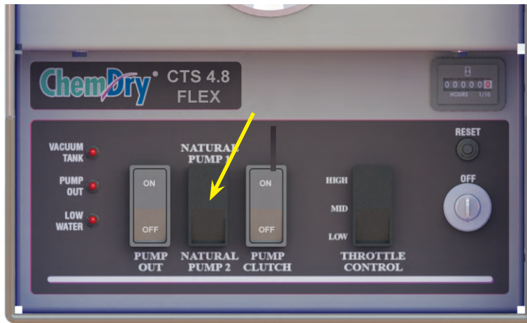
Figure 2-9. Press NATURAL PUMP Switch to Middle “OFF” Position
