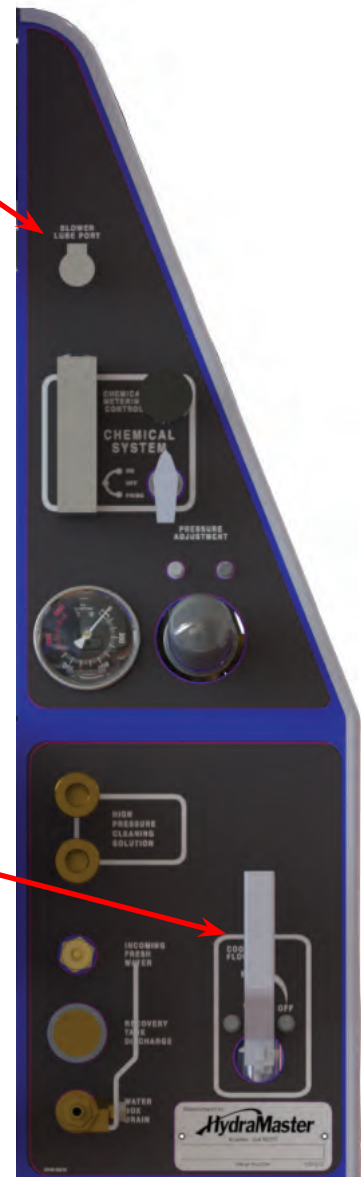
Figure 2-3. CTS 4.8 Flex Instrumentation Panel
