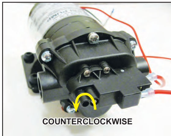
Figure 9-11. Insert Hex L-Key and Turn It Counterclockwise/Clockwise
