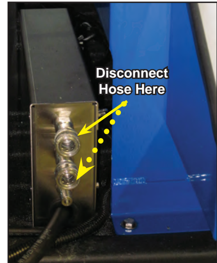
Figure 9-9. Disconnect Solution Hose
