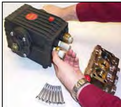
Figure 4-7. Seal Assemblies May Come Off with Manifold
