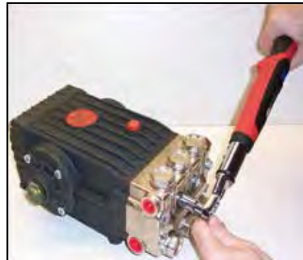
Figure 4-18. Torque Bolts to 22 ft.-lbs (3 m-kgs)
