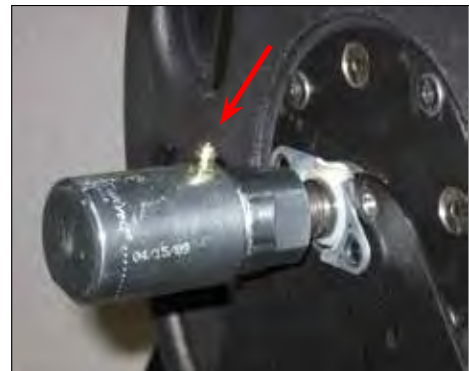
Figure 8-2. Location of Zerk on Swivel
