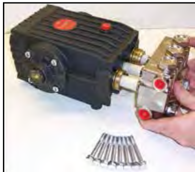
Figure 4-7. Seal Assemblies May Come Off with Manifold
