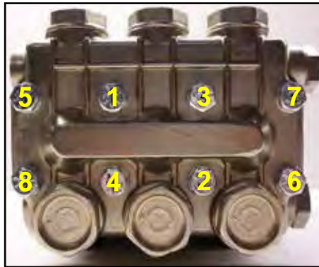
Figure 4-17. Torque Sequence in "X" Pattern
