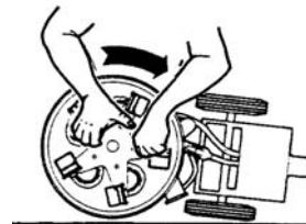
Figure 6-2. Remove Cleaning Head
