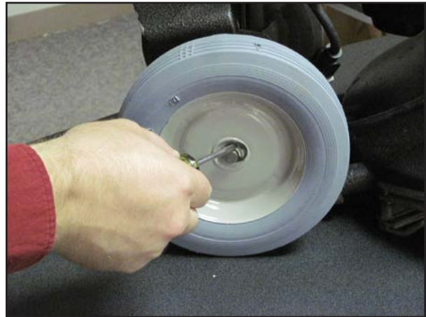
Figure 6-6. Remove Retaining Clip with Screwdriver
