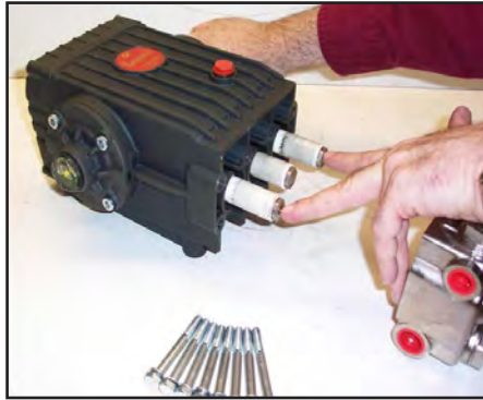
Figure 6-16. Re-install Manifold and Torque Fasteners
