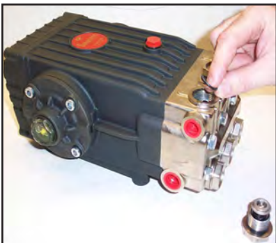
Figure 6-4. Apply Grease and Install Valves
