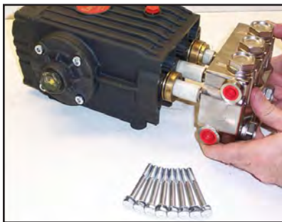
Figure 6-7. Seal Assemblies May Come Off with Manifold
