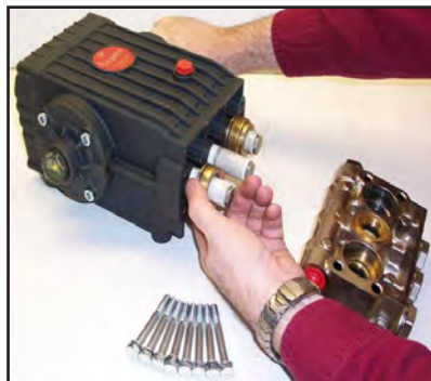
Figure 6-7. Seal Assemblies May Come Off with Manifold
