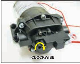
Figure 4-5. Insert Hex L-Key and Turn It Counterclockwise/Clockwise
