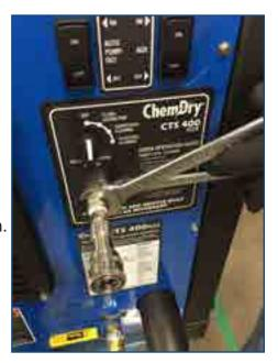
Figure 4-6. Remove Quick Connect Assembly
