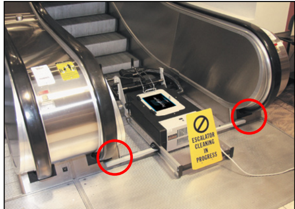
Figure 5. Ensure Restraining Arms are Firmly Seated Against Balustrades
