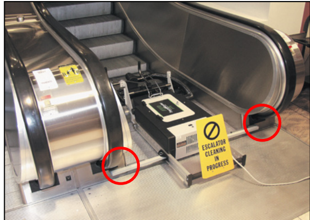
Figure 12. Ensure Restraining Arms are Firmly Seated Against Balustrades
