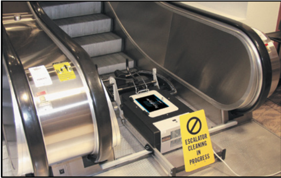
Figure 9. TreadMaster Shown in Preferred Placement, at Bottom of Escalator
