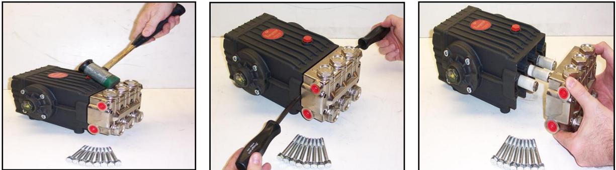
Figure 7. Separate Manifold from Crankcase
