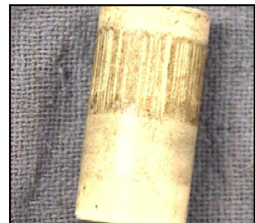
Figure 6. Examine Ceramic Plungers
