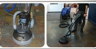
8 For grout, it is important to neutralize the cleaning solution residue. Mix 1 part HydraStone with 32 parts water and apply to grout. Allow several minutes of dwell time and then rinse with water.
