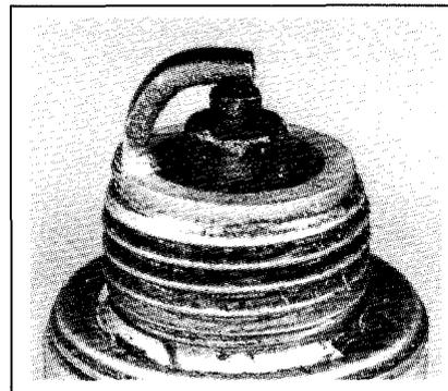
**Wet Fouled:** A wet plug is caused by excess fuel, or oil in the combustion chamber. Excess fuel could be caused by operating the engine with too much choke. Oil in the combustion chamber is usually caused by worn piston rings or valve guides.
