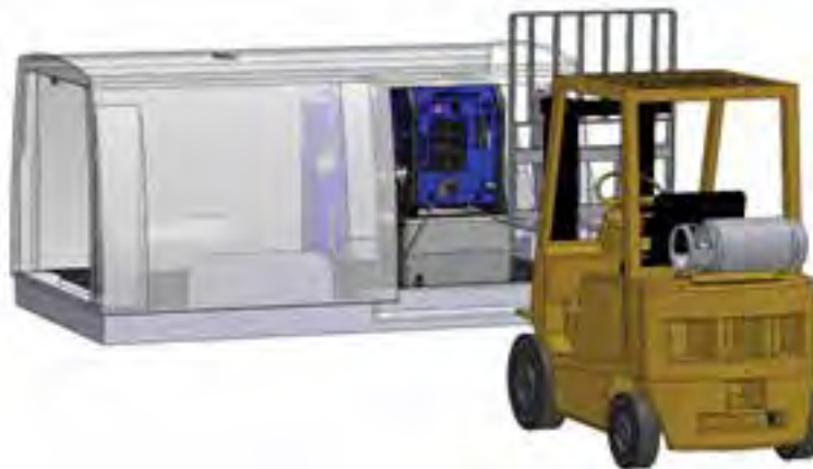
Figure 2-3. Use Forklift to Position Machine
