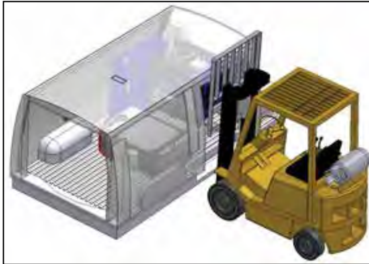
Figure 2-2. Load FWT into Vehicle until Truckmount Is In Place
