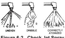
Figure 6-2. Check Jet Spray for Even Flow
