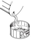
Figure 9-2. Use Can to Hold Oil for Seal
