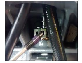
Figure 9-5. Reinstall dog point set screw
