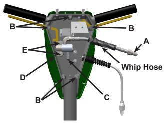
Figure 9-3. Valve Assembly Parts
