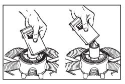
Figure 6-6. Lubricate Vacuum Seal on Top of Hub
