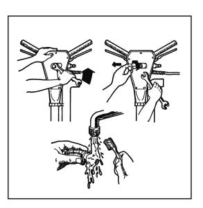
Figure 6-1. Remove Nut/Inline Filter
