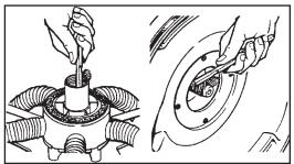
Figure 6-5. Clean Off Debris from Gear Box Shaft
