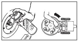
Figure 6-7. Lubricate Shaft and Re-install Head Assembly
