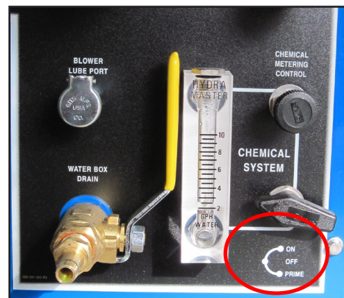
Figure 4-7. Location of Chemical System Switches
