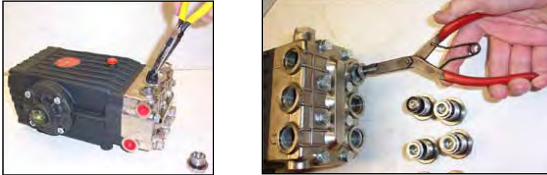
Figure 5-1. Remove Valve Cap and Valve Assembly
