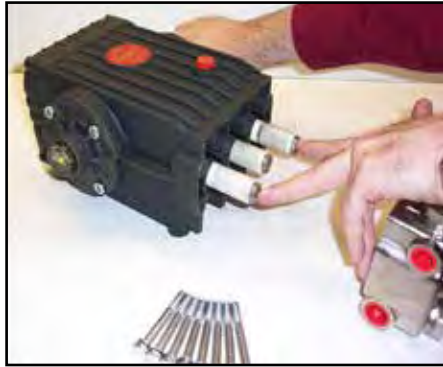
Figure 5-16. Re-install Manifold and Torque Fasteners
