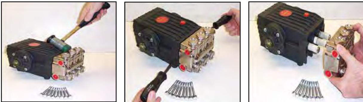
Figure 5-6. Separate Manifold from Crankcase
