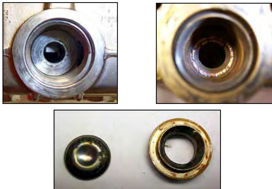
Figure 5-2. Inspect Manifold and Old Valves
