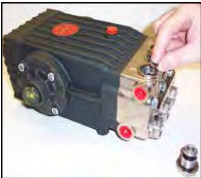
Figure 5-4. Apply Grease and Install Valves
