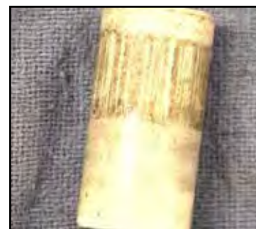
Figure 5-8. Examine Ceramic Plungers
