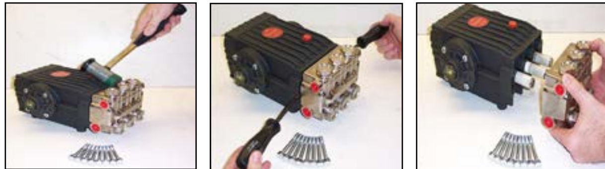
Figure 5-6. Separate Manifold from Crankcase
