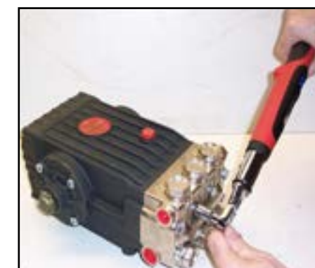
Figure 5-18. Torque Bolts to 22 ft. lbs
