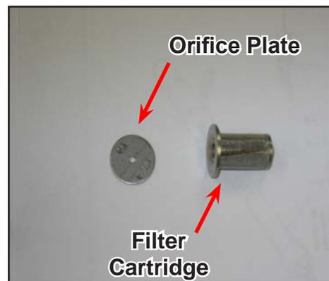
**Figure 3-8. Remove Filter Cartridge and Plate Orifice**
