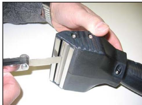
**Figure 3-6. Clean the Solution Bar Jet**
