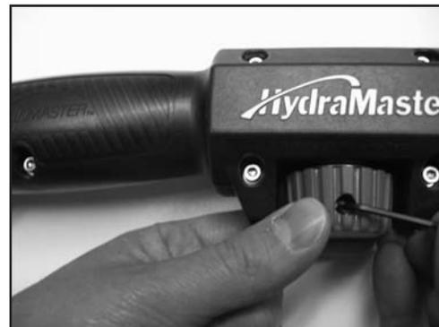
**Figure 3-2. Remove Solution Control Knob**
