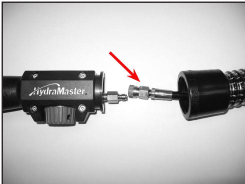
Figure 3-1. Remove Tool from Hose
