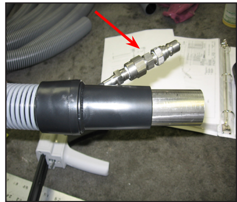
Figure 3-7. Disassemble Solution Quick Connect
