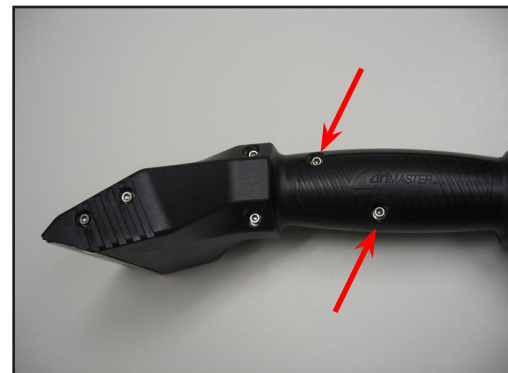
Figure 2-1. Remove Tool Screws
