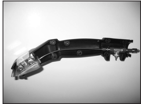
Figure 3-5. Re-install Clear Window Cover
