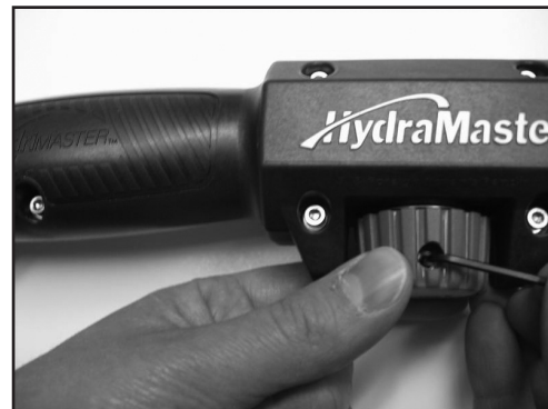
Figure 3-2. Remove Solution Control Knob
