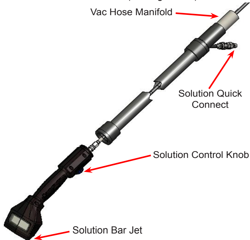
Figure 2-3. Attach Solution Hose and Adjust Water Volume
