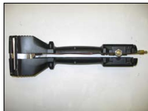
Figure 3-4. Separate Cover Halves
