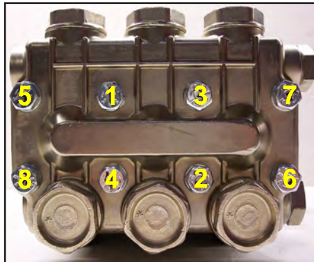
Figure 5-17. Torque Sequence in “X” Pattern
