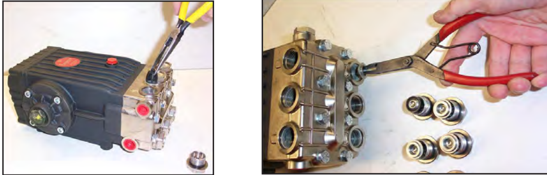
Figure 5-1. Remove Valve Cap and Valve Assembly
